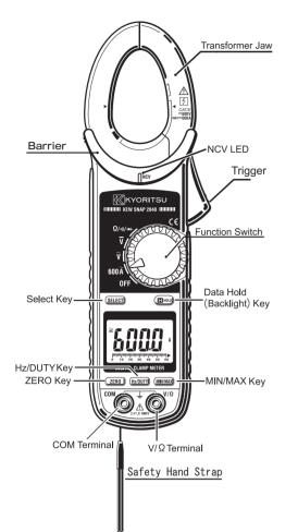
Barrier : It is a part providing protection against electrical shock and ensuring the minimum required air and creepage distances.
